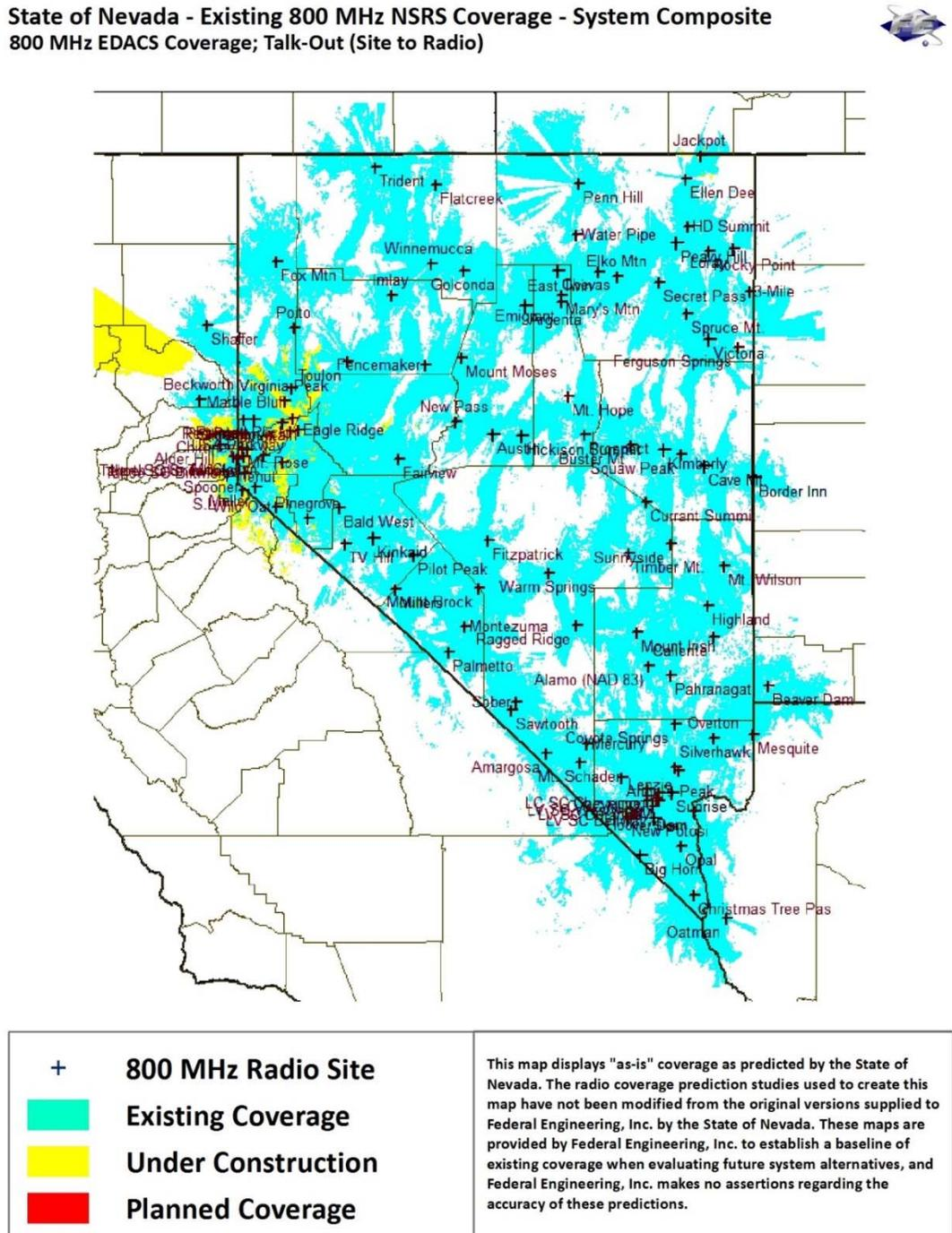
**Figure 5 – Existing 800 MHz NSRS Mobile Radio Talk-out Coverage from all stakeholder sites**
