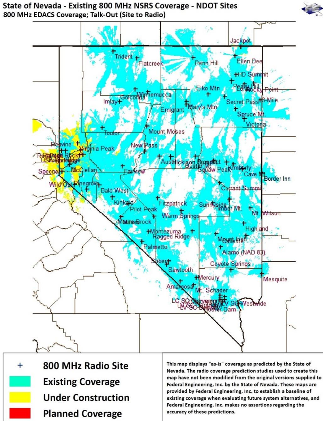
**Figure 2 – Existing 800 MHz NSRS Mobile Radio Talk-out Coverage from NDOT sites**
