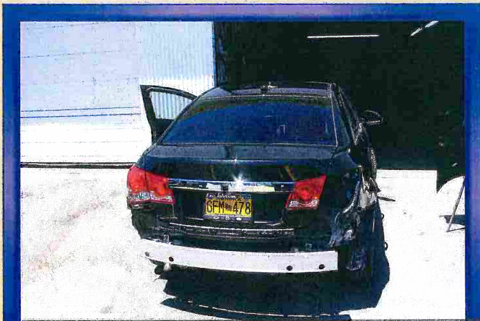
Freshly painted rear bumper, right rear quarter panel & trunk lid area.
