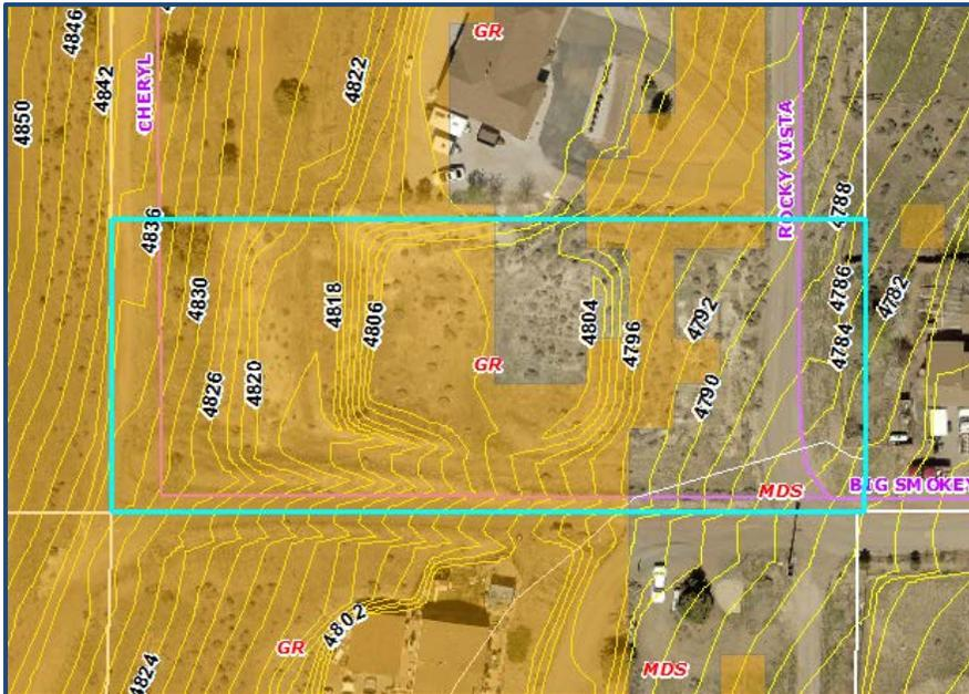
**Slopes and contours of subject parcel. The orange shading represents slopes between 15-30%. Below is a graphic illustrating the existing easement and proposed reduction.**
