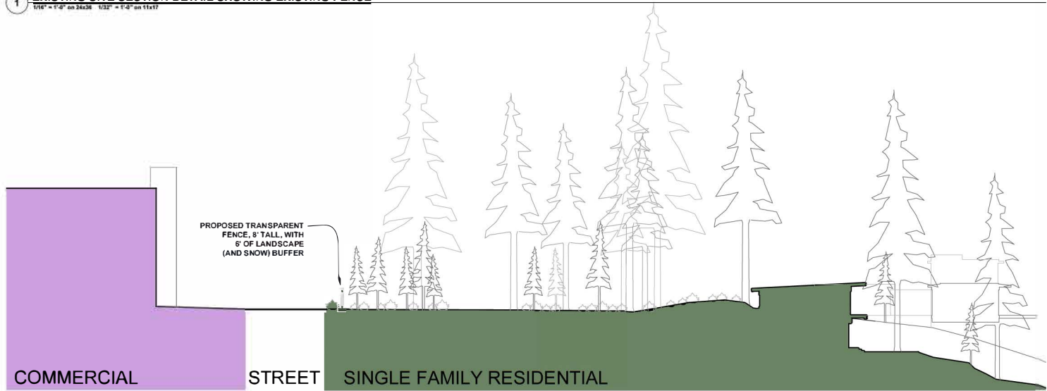
2 SITE SECTION DETAIL SHOWING PROPOSED FENCE & LANDSCAPE BUFFER 1/16" = 1'-0" on 24x36 1/32" = 1'-0" on 11x17
