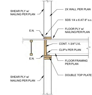
JOISTS BOTH DIRECTIONS w/ SHEAR WALL
