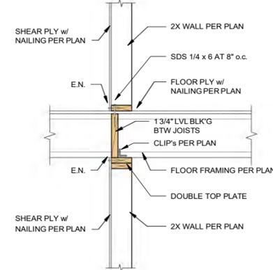
JOISTS PERPENDICULAR w/ SHEAR WALL
