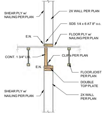
JOISTS PARALLEL w/ SHEAR WALL
