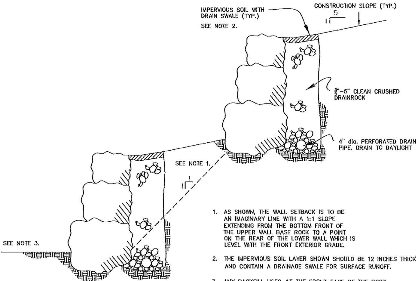
1. AS SHOWN, THE WALL SETBACK IS TO BE AN IMAGINARY LINE WITH A 1:1 SLOPE EXTENDING FROM THE BOTTOM FRONT OF THE UPPER WALL BASE ROCK TO A POINT ON THE REAR OF THE LOWER WALL WHICH IS LEVEL WITH THE FRONT EXTERIOR GRADE.
