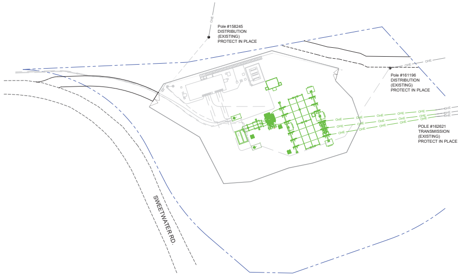
PHASE B - REMOVAL / DEMOLITION IN 2027 (IN GREEN)
