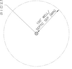
ESTIMATED PRIMARY LEACH FIELD TRENCH LOCATIONS, MINIMUM 100' FROM ANY DOMESTIC WATER WELLS. (DESIGN BY OTHERS AND UNDER SEPARATE PERMIT)
