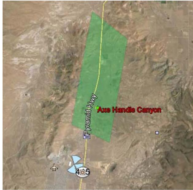
The search ring represents the area within which a facility can be located to achieve the desired coverage objective. The centerline height of 100' represents the required height of the antennas to produce the desired coverage. After reviewing the County's zoning regulations, the next step is to identify any existing towers within the search ring that could allow for co-location.
