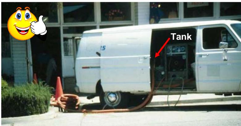
**Figure IC-17.** The photograph above demonstrates good storm water management practice. This mobile carpet cleaning operation is pumping and containing used wash water in a tank located inside the van. The used wash water is later discharged to a RV dump station or to the sanitary sewer system for proper disposal. (Source: CASQA).
