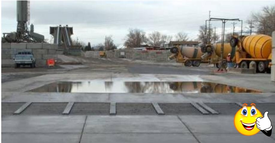
**Figure IC-8a.** The photograph above demonstrates good storm water management practices at a fixed facility. A tire wash at a local concrete ready-mix operation reduces track out of sediment and concrete waste onto paved roadways. (Source: Sparks Environmental Control)
