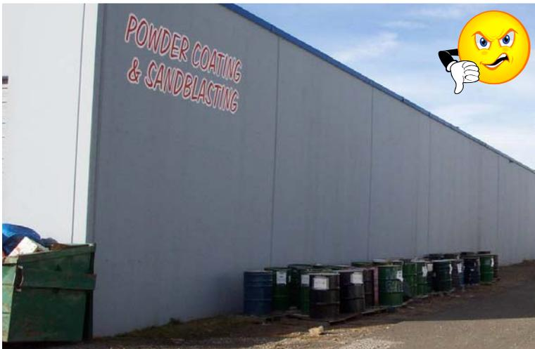
**Figure IC-3c.** The photograph above demonstrates poor storm water management practices. These drums should be stored under cover or indoors to prevent interaction with storm water (Source: Sparks Environmental Control).
