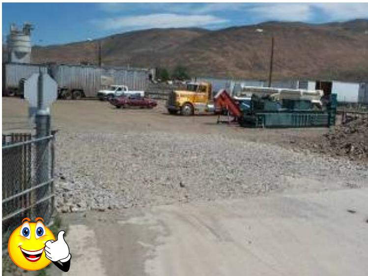
**Figure SC-1a.** The photograph above demonstrates a storm water BMP. The entrance/exit at this facility has been stabilized with rock to reduce the tracking of sediment from the dirt lot onto paved roadways. (Source: Sparks Environmental Control)
