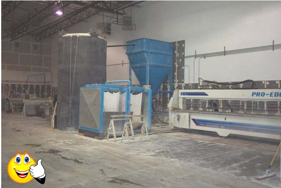
**Figure IC-7c.** The photograph above demonstrates good storm water management practices. This indoor granite/stone cutting facility uses proper filtering and ventilation to prevent the escape of dust. It also recycles all of its process water, having no discharges to the sanitary sewer or storm drain systems (Source: Sparks Environmental Control).
