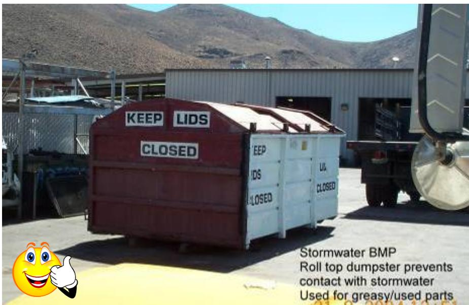
**Figure IC-1c.** The photograph above demonstrates good storm water management practices. Used vehicle parts are being properly stored for disposal in a covered dumpster. (Source: Sparks Environmental Control)
