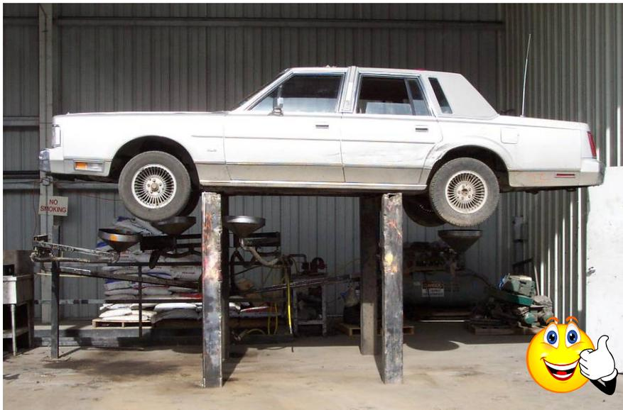
**Figure IC-5d.** The photograph above demonstrates good storm water management practices. All fluids should be drained from vehicles upon arrival at the facility and before storage (Source: Sparks Environmental Control).
