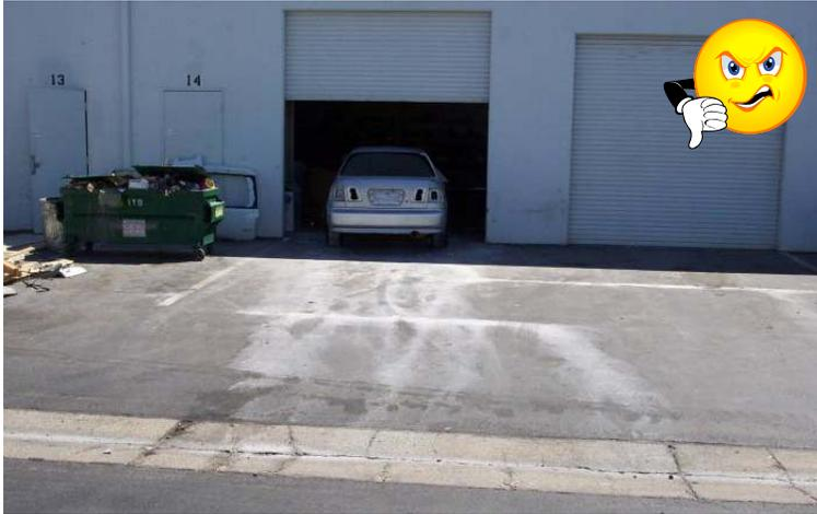
**Figure IC-3b.** The photograph above demonstrates poor storm water management practices. Sanding / body work waste from an auto body repair shop is draining into a valley gutter and into the storm drain system (Source: Sparks Environmental Control).
