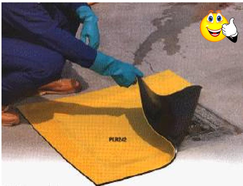
**Figure IC-15b.** The photograph above demonstrates a storm water BMP. A storm drain cover such as this can be used to seal off storm drains in the vicinity during washing activities. (Source: Kevin P. Walker, C&S Engineers, 2005)
