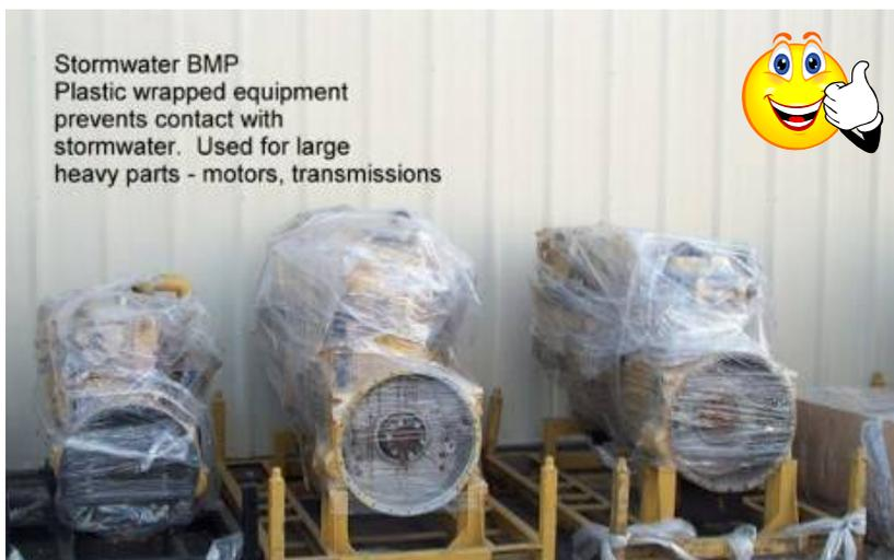
**Figure IC-1a.** The photograph above demonstrates good storm water management practices. This local vehicle repair facility is properly storing vehicle engine components outdoors. (Source: Sparks Environmental Control)
