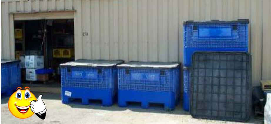
**Figure IC-5a.** The photograph above demonstrates good storm water management practices. Used batteries and brake shoes should be properly stored in covered containers. (Source: Sparks Environmental Control)
