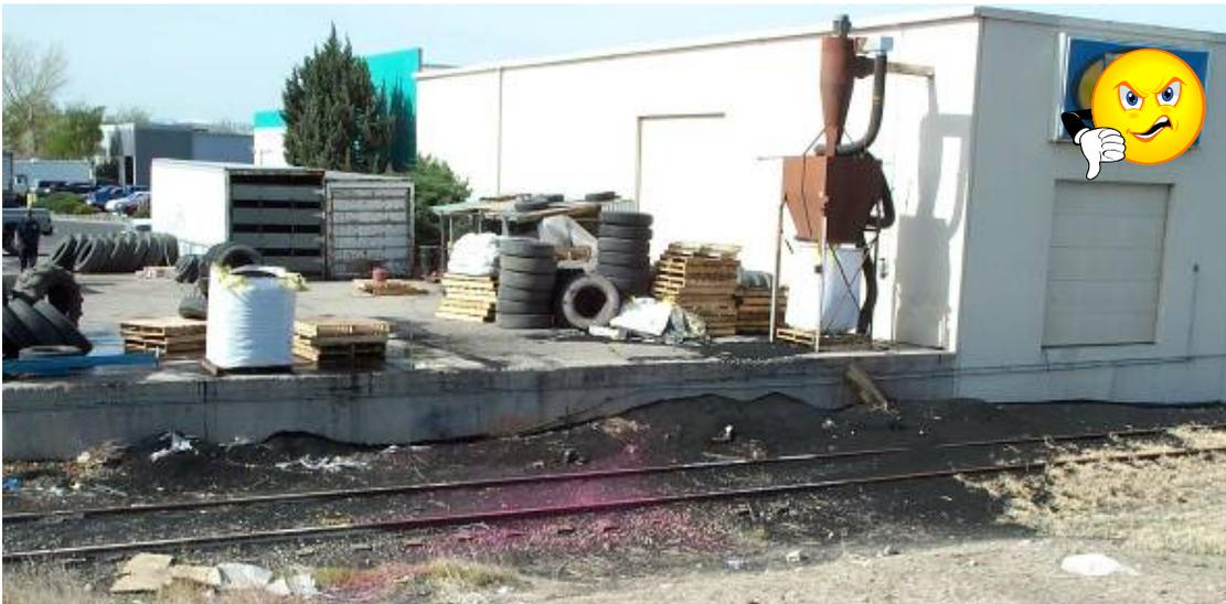
**Figure IC-5b.** The photograph above demonstrates poor storm water management practices - uncontained rubber and metal waste material from a tire re-treading facility has been allowed to accumulate in an exposed outdoor area. This waste is exposed to storm water and could become pollutants that discharge to the river. (Source: Sparks Environmental Control)
