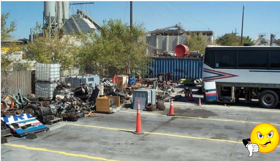
**Figure IC-1e.** The photograph above demonstrates poor storm water management practices. Uncovered and uncontained used engine parts at this site are leaking petroleum hydrocarbons and other pollutants onto the ground which will eventually discharge to the storm drain system. (Source: Sparks Environmental Control)
