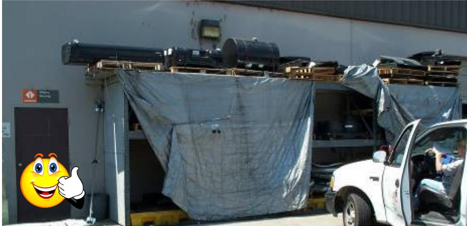
**Figure IC-1b.** The photograph above demonstrates good storm water management practices. Used batteries and brake shoes are being properly stored in covered shelving with containment pallets to capture any spills. (Source: Sparks Environmental Control)
