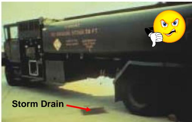
**Figure IC-14b.** The photograph above demonstrates a poor storm water management practice. This fuel tanker truck is parked directly over a storm drain inlet. Mobile fueling vehicles such as this should be parked at least 50 feet from the nearest storm drain. (Source: Air Force Center for Environmental Excellence).
