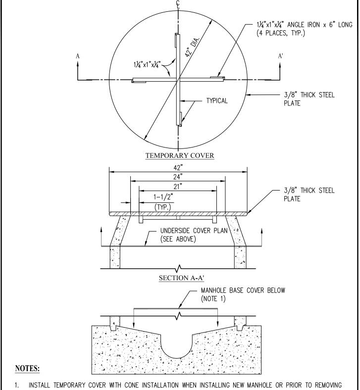
EXISTING FRAME & COVER AND GRADE RINGS TO ADJUST TO FINISH GRADE. INSTALL COVER OVER MANHOLE BASE TO PREVENT DEBRIS FROM ENTERING SEWER SYSTEM. THE MANHOLE BASE COVER SHALL BE IN PLACE PRIOR TO PERFORMING ANY ADJUSTMENTS OR GROUTING AND SHALL REMAIN IN PLACE WHILE ADJUSTMENTS OR GROUTING ARE BEING PERFORMED. REMOVE BASE COVER UPON ADJUSTMENT APPROVAL BY WASHOE COUNTY.
