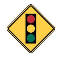
ASWS include the yellow signs stationed over the roadway that often feature flashing yellow lights to warn of a traffic signal ahead.
