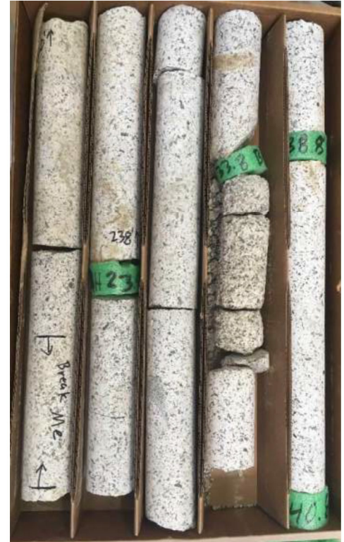
Granitic Bedrock Cores Boring B-09, 20.5 to 40.8 Feet
